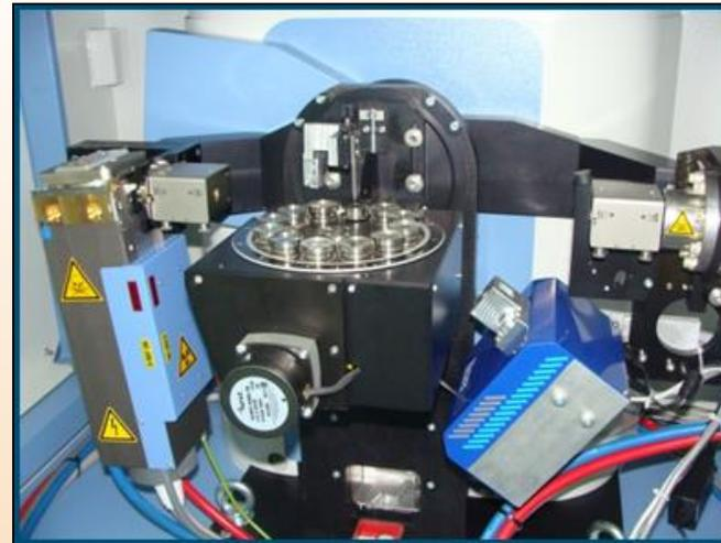
The measuring part consisting of X-ray tube, the automatic feeder and two detectors
