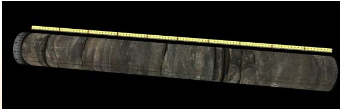
3D photo of sidewall surface of drill core, 1 meter
