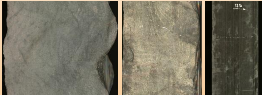
Sidewall surface of unrolled core samples
