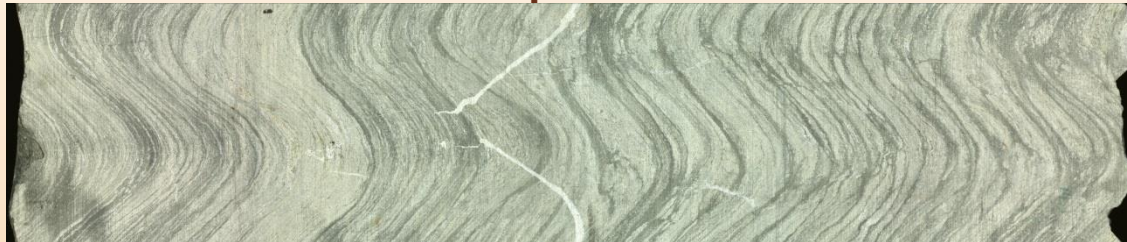
Sidewall surface of unrolled drill core, 1 meter long
