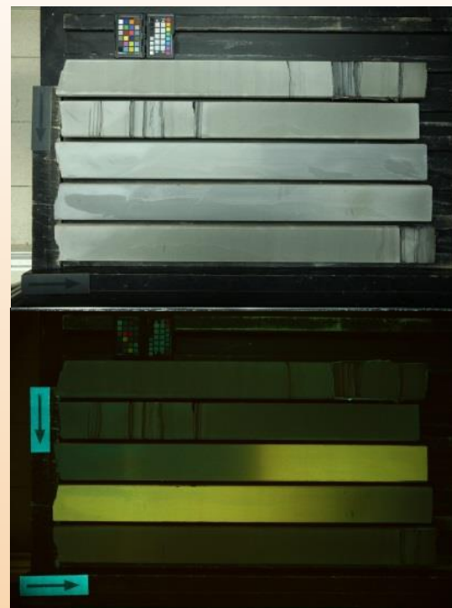
Photo of whole core lighted by natural daylight and ultraviolet light
