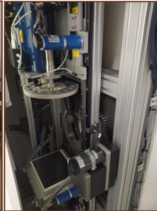
The rotating “source- detector” system
