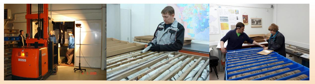
The core arriving from subsoil users in process of preparation for long-term storage is submitted to thorough examination, where necessary immediate core study is conducted, and then it is placed in a special container and placed directly in cells of racks.
